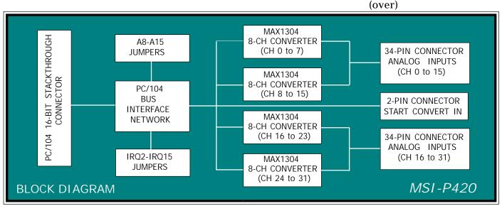
Channels for each of four devices can be enabled or disabled via the configuration register of the devices. Conversion times of approximately 800ns to 2200ns for 1 to 8 channels, respectively, for each device. Since conversions are simultaneous, all four devices are converting at the same time for a maximum time of approximately 2200ns for all 32 channels.
