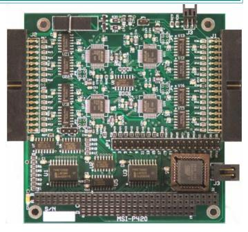
with capacities of 8, 16, 24 or 32 channels with a non-linearity of  $\pm 1/2$  LSB. The card operates from a single +5V supply and the inputs are overvoltage tolerant to  $\pm 9V$ . A block diagram of the card is shown in Fig. 1.
